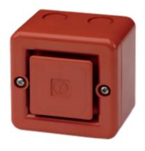
The EXS230-1 is a compact, high output, 100dB(A) alarm sounder. Low current consumption and high SPL in a robust fire retardant housing ensure the EXS230-1 is suitable for all general signalling applications including fire, security and process control.
