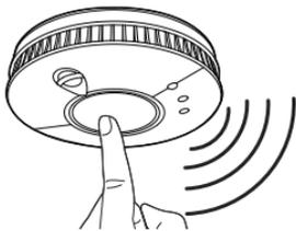
During these five seconds you need to briefly press the test button on Alarm 1 to wirelessly interlink the two alarms. Alarm 1 will give an audible sound consisting of two cycles of three loud beeps.
