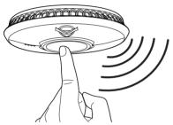
**b** Your alarm will silence and enter into a reduced sensitivity reset cycle for approximately 10 minutes.
