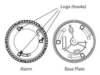
There are three lugs (hooks) on the back of the alarm that slide in to three slots on the base plate. The alarm can be attached in any orientation, simply line up the lugs (hooks) with the holes at the end of the slots then twist the alarm clockwise until the alarm stops, make sure the alarm is twisted on fully.
