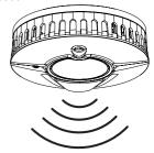
b The unit's Escape Light will illuminate and it will sound an audible alarm consisting of 2 cycles of 3 loud beeps, then stop automatically.
