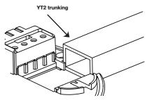
Either feed the wire through the hole in the base plate or through the YT2 trunking.
