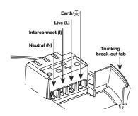
**WARNING:** Mixing the Live and Neutral connections when interconnecting alarms will damage all the alarms. DO NOT use the Earth wire for the interconnect connection.
