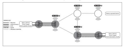
**Make sure there is only one wireless connection into each wired network.** For example if you have a hardwired network upstairs and a wireless network downstairs only one of the hardwired products should be linked into the wireless network, connecting both systems.
