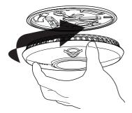
Once the smoke alarm has been fitted onto the base plate correctly, the internal power pack will activate. The red LED on the front of the alarm should now flash once every 40 seconds to show that it is active.
