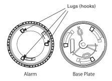
When used with the base plate, the alarm can be attached in any orientation, simply line up the lugs (hooks) with the holes at the end of the slots then twist the alarm clockwise until the alarm stops, make sure the alarm is twisted on fully.
