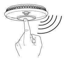
**b** Your alarm will silence and enter into a reduced sensitivity reset cycle for approximately 10 minutes.
