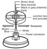
If desired, the alarm can be interconnected with up to 11 other smoke (SW1), heat (HW1) or carbon monoxide (CW1) alarms from the FireAngel range via the 'I' connector. (See Optional Interconnecting Feature)
